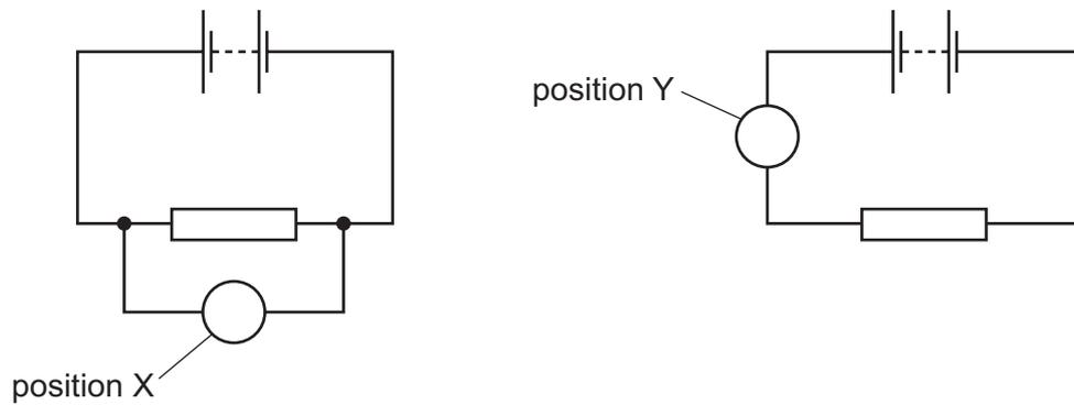
What meter is used, and where is it connected in the circuit?
